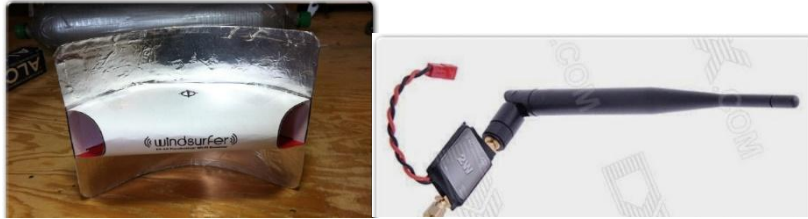
Fig. 1. a. Parabolic reflector. b. Intermediate amplifier[10]
