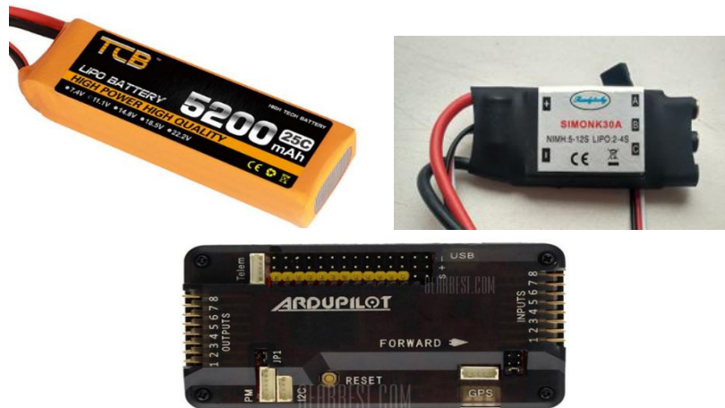
Fig. 11. a. Rechargeable batteri, b. Speed regulator Simonk 30 A speed controller is a programmable controller, c. APM2.8
