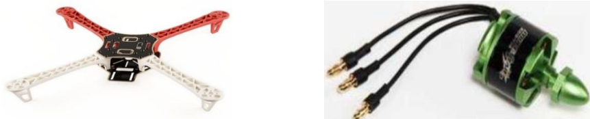
Fig. 10. a The frame is made of plastic, but my rigid characteristics b. Collectorless motors
