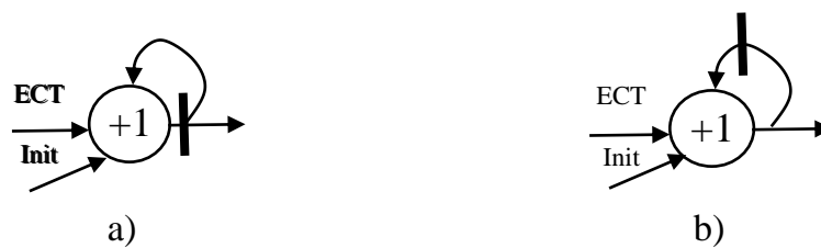
Fig. 1. Counter model with output from the register (a) and from the node (b)
